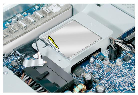
6. Reconnect the antenna cable to the hole on the AirPort card guide.
